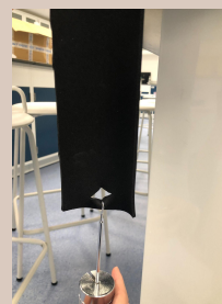
Fig.28 Neoprene fabric break during testing
